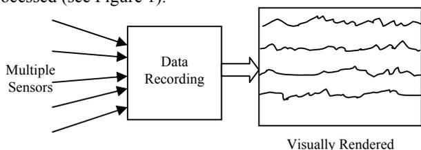
Figure 1: System diagram showing current visual analysis of gathered data
