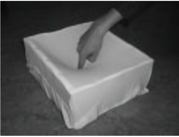
Fig. 1. The InvisiBall. Finger position in the 3D space is detected in real-time.
