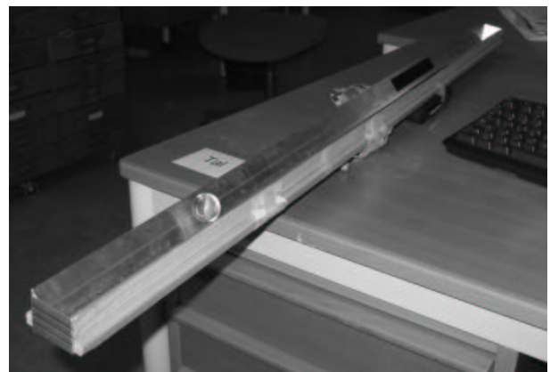
Fig. 2. The "rolling-track" with a glass marble rolling in its upper-face aluminium track.
