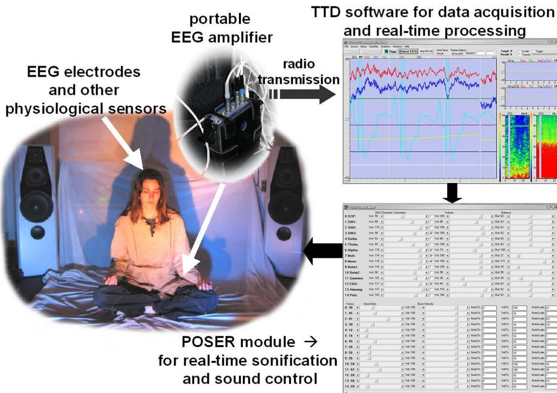
Figure 1: Feedback setting of an interactive ‘brainmusic’ concert. The performer wears a portable EEG amplifier that sends the signal wirelessly to the TTD software. The TTD performs real-time filtering and other signal processing and sends the data to the POSER module for sonification. The sonified signals are presented over loudspeakers so that the performer can interact with the sound of its own body.
