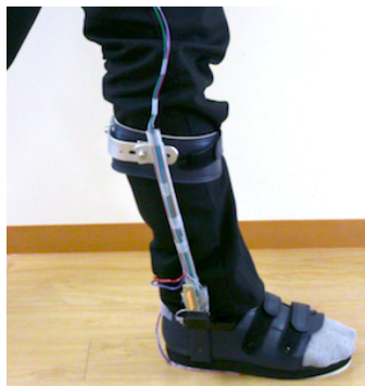
Figure 2: A picture of the ankle-foot orthosis (AFO). The angle of ankle joint was measured by a goniometer and sent to a PC via Bluetooth serial communication.
