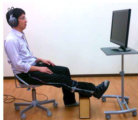
Figure 1: A picture of the experimental set-up and instrumentation. Participants were asked to perform voluntary ankle dorsi-plantarflexion movements.
