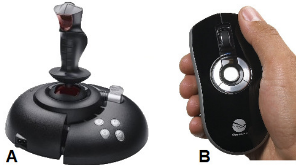
Figure 8. Microsoft’s Sidewinder “Force Feedback 2” joystick, and Gyration’s “Air Mouse”.
