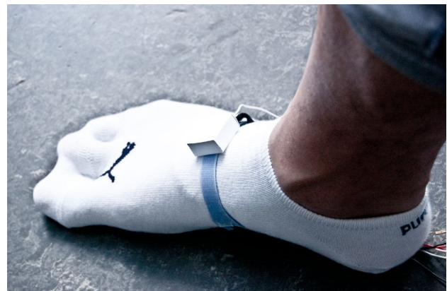
Figure 1. Foot-glove and a cased accelerometer, which is part of the IMU-motion capture system
