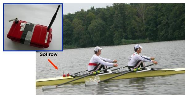
Figure 1: *The training and measurement system Sofirow (developed by BeSB GmbH Berlin and University of Hamburg) located on top of the JM2x.*
