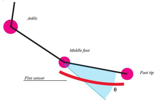
Figure 4. The flex sensor linear readings interpreted as 2D rotation angle( $\Theta$ ) affecting  $T$ (footTip) and  $A$ (middleFoot) vectors
