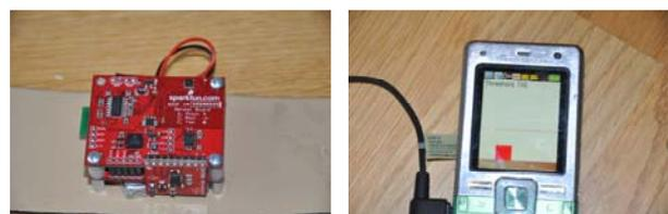
**Figure 2.** The sensor (left image) used in this experiment. It is a 6DOF (Sparkfun Inc.) inertial measurement unit with Bluetooth antenna. The telephone (Sony Ericsson 650i) received the data via Bluetooth, computed vertical displacement and step frequency and presents the information visually (right image) and via an auditory display.
