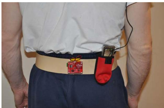
**Figure 3.** The system worn by a runner. The sensor is securely attached to a belt. In this case, the user has an earphone attached to the phone via cable. Of course, a bluetooth headset would work as well. As there is no cable between the sensor and the phone, the user does not need to carry the phone when the running takes place on a treadmill.
